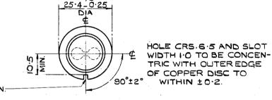
OF COPPER DISC TO WITHIN ±0.2. ACCEPT 16" DIA PIN-
