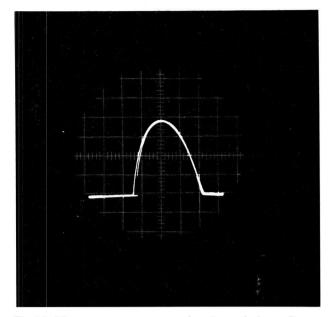
Fig. 11 RF power output as a function of the reflector voltage. The oscillogram shows the low hysteresis when the reflector voltage is wobbled as a difference in RF output at increasing and decreasing reflector voltage.
