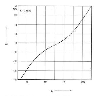
Fig. 9 Modulation characteristic of the **TK 6**
