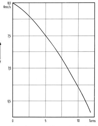
Fig. 3 Klystron frequency as a function of the number of turns of the tuning screw
