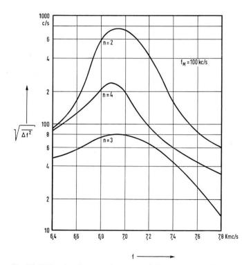
Fig. 14 Noise level as a function of frequency for the modes n = 2,3,4
