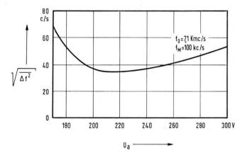
Fig. 13 Noise level as a function of acceleration voltage
