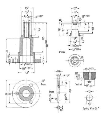
Fig. 5 Components of waveguide coupling
