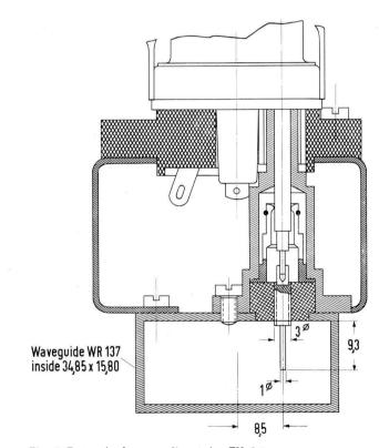
Fig. 4 Example for coupling tube **TK 6** to a square waveguide
