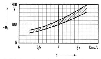
Fig. 7 Optimum reflector voltage as a function of frequency
