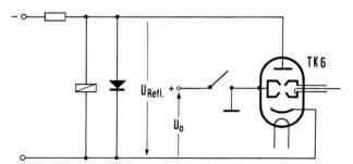
Fig. 15 Proposed circuit for the automatic disconnection of the resonator voltage when there is no, or a positive, reflector voltage
