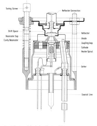
Fig. 2 Design of the Reflex Klystron TK 6
