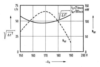
Fig. 12 Noise level and RF energy as a function of reflector voltage
