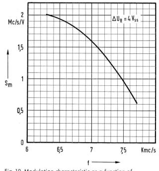
Fig. 10 Modulation characteristic as a function of frequency
