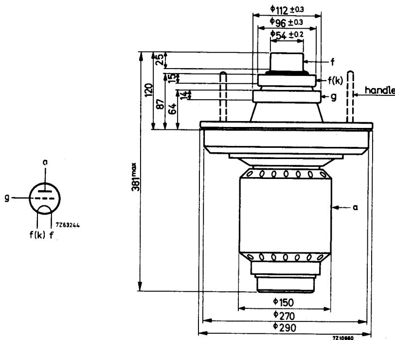
Note: The handles should be removed before switching on the tube.
