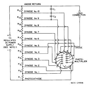
$C_1$ : 0.02  $\mu$ F, 20%, 500 volts (dc working), ceramic disc  $C_2$ : 0.01  $\mu$ F, 20%, 500 volts (dc working), ceramic disc  $R_1$ : 910,000 ohms, 2 watts
