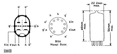
The triode on pins 6, 7, 8, 9 should have grounded-cathode connection and that on pins 1, 2, 3 should have grounded-grid connection.
