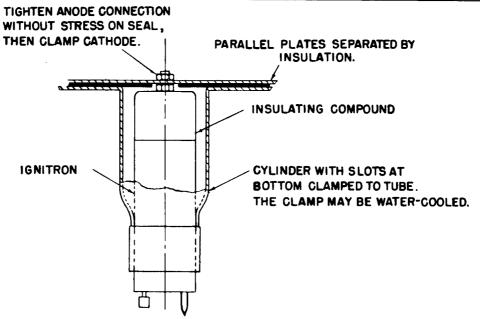
SUGGESTED METHOD FOR PROVIDING MOUNTING FOR COAXIAL CONNECTION
