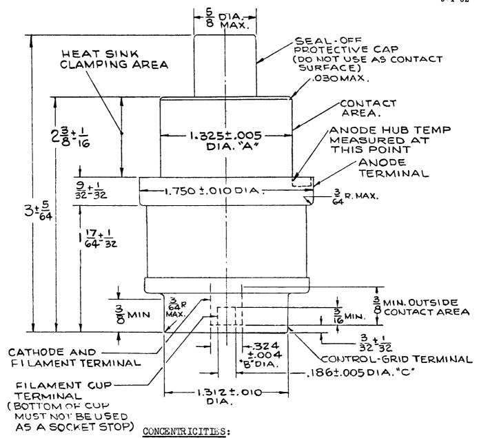
The following total indicator readings are measured with respect to a centerline determined by the centers of the anode terminal and control grid terminal.
