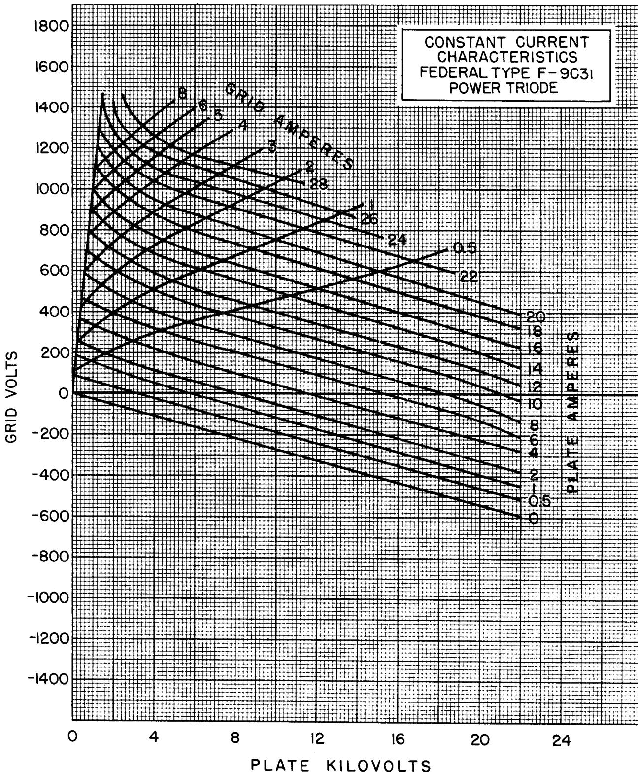
In Federal's latest 50 Kilowatt A.M. Transmitter, the F-9C31 is used in the R.F. Amplifier, the F-9C29 in the Modulator.
