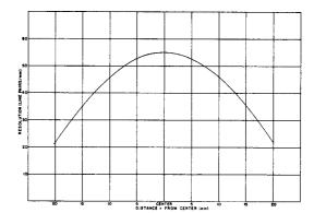
Characteristic resolution curve with tube immersed symmetrically in cylindrical solenoid (uniform winding) and focused for maximum resolution in center of field. Dimensions of solenoid: 7½ inches long, 9½ inches OD, 4¾ inches ID.
