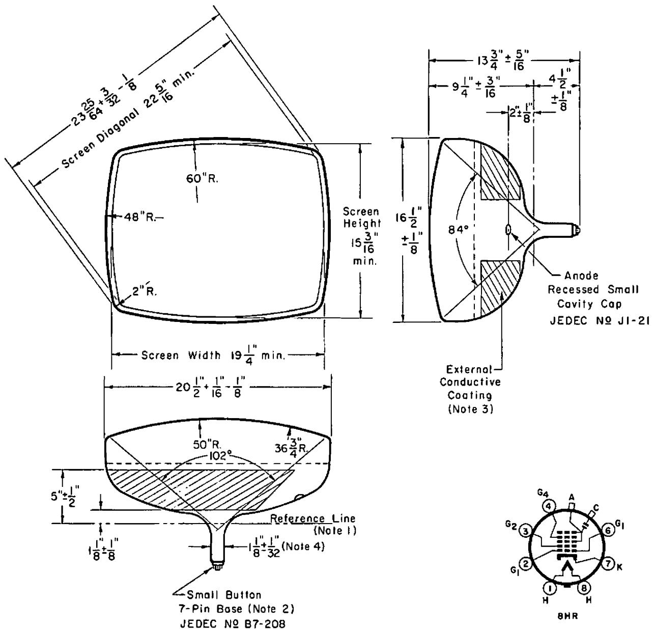
**NOTE 1:** Yoke Reference Line is determined by plane surface of flared end of JEDEC Reference-Line Gauge No. 126 when seated on funnel of tube. With a minimum neck length tube, the PM centering magnet (0 to 8 gauss) should extend no more than  $2\frac{1}{8}$  from Yoke Reference Line.
