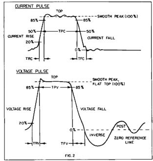
No spike or ripple shall exceed  $\pm$  7% of the average peak value of voltage or current. Inverse voltage should not exceed 20% of the forward voltage. Post voltages should be held to a minimum as they may cause post pulse noise or oscillation.
